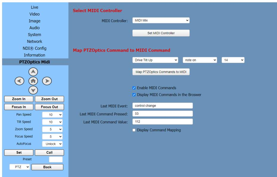
photo (left), you can see that the **Drive Tilt Up** command would be mapped to the **Note On** event from **MIDI Command 14**.
